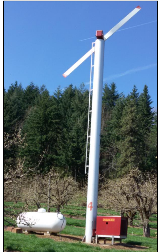
Frost fan tower with blades, engine and propane tank (Photo: Lesley Tamura)
