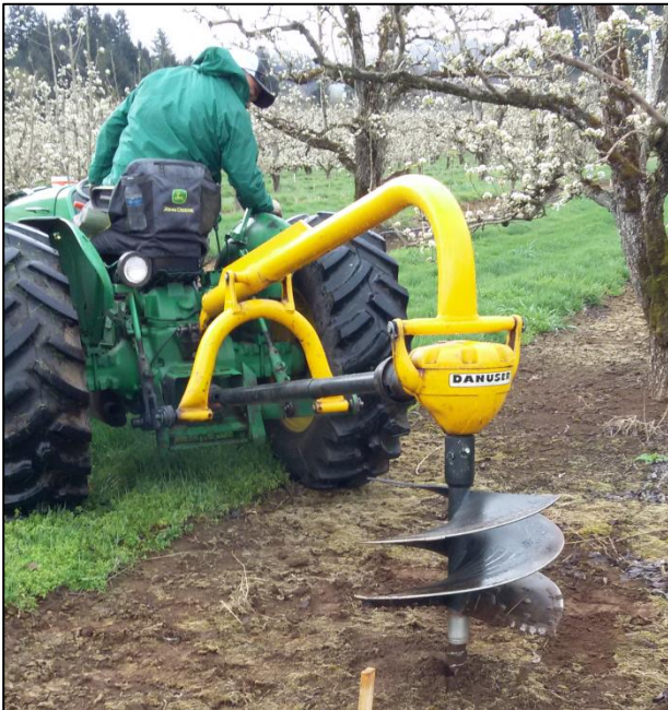
Large drill attached to a tractor for digging tree holes (Photos: Lesley Tamura)
