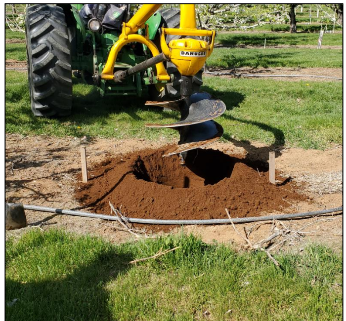
Large drill attached to a tractor for digging tree holes (Photos: Lesley Tamura)
